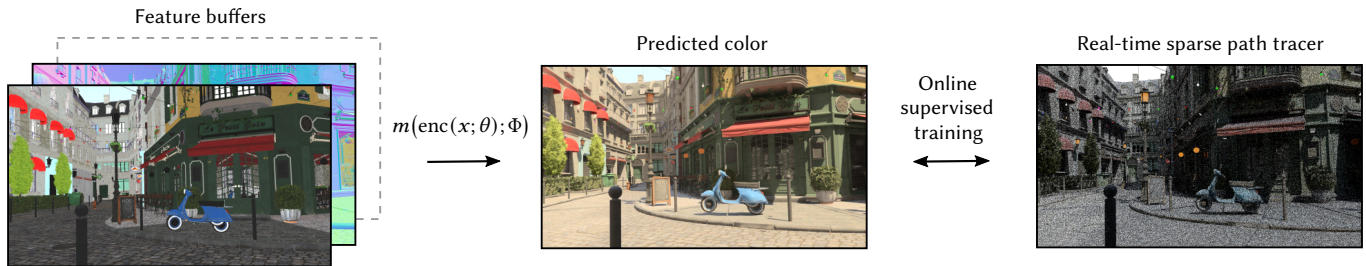
Fig. 8. Summary of the neural radiance caching application [Müller et al. 2021]. The MLP m(\text{enc}(x; \theta); \Phi) is tasked with predicting photorealistic pixel colors from feature buffers independently for each pixel . The feature buffers contain, among other variables, the world-space position x , which we propose to encode with our method. Neural radiance caching is a challenging application, because it is supervised online during real-time rendering . The training data are a sparse set of light paths that are continually spawned from the camera view. As such, the neural network and encoding do not learn a general mapping from features to color, but rather they continually overfit to the current shape and lighting. To support animated content, training has a budget of one millisecond per frame .
